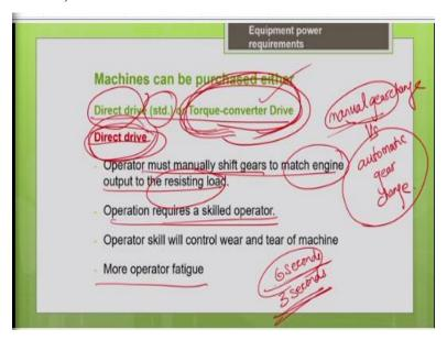
So, another important thing to be noted is the machines when you purchase depending upon the mode of transmission, you can call it as direct drive base machine or torque converted drive-based machine. In a simple way to say it is nothing but your manual gear change versus automatic gear change. So, basically your direct drive is nothing but your manual gear change.
