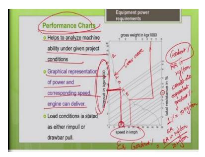
So, you have to draw a vertical line intersecting your total resistance percentage line. Once it intersects your; the total resistance percentage line, then draw a horizontal line to the left intersecting your gear curve. Now drop a vertical line intersecting your speed, so this is how you can find the speed of the machine if you know the total resistance percentage.
