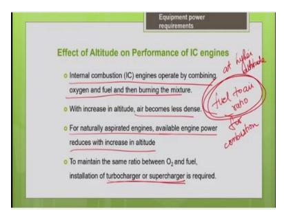
Now let us see what is the effect of altitude on the performance of the engine? So, as we discussed earlier, the usable power depends upon the underfoot conditions, altitude and temperature. So, you know that the horsepower rating of the machine is done with the standard conditions by the manufacturer. So, they might have done the horsepower rating at standard temperature and the standard atmospheric pressure.
