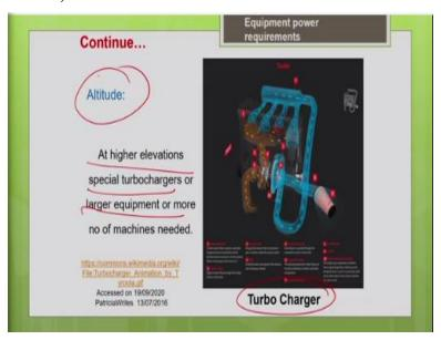
So, I have shown you this picture in the lecture 1, hope you remember, like you can see this blue color indicates the air movement, there will be a compressor arrangement, which will compress the air and supply the air and maintain the air to fuel ratio in the chamber. So, that is how the combustion process is not effective, if you provide this the turbocharger. So, at higher elevations either you should go for these kinds of special turbochargers.
