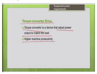
So, other one as we discuss just now is torque converter drive, it is initial cost is high. So, you have a torque converter device here which can automatically match your adjust your power output to match the load conditions, so it results in higher productivity. So, you know why higher productivity because your maneuver time is going to be lesser here, your cycle time will be reduced, so the productivity will increase.
